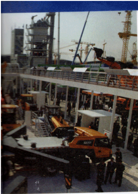
The Sany STC2200 is a 200 tonne capacity truck crane on a five axle carrier
