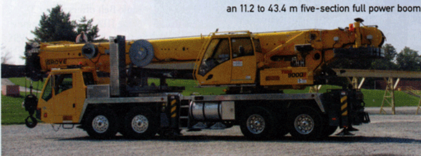
The 90 tonne capacity Manitowoc Grove TMS9000E has an 11.2 to 43.4 m five-section full power boom
